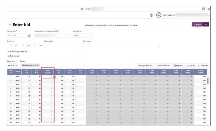
For BDUs, the recall period column is added to both the LOAD and GEN sides.
